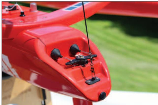
*The pushrods for the rudder exit the hull through water resistant boots, further helping to keep water out.*
