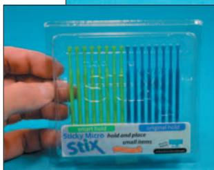
Left: Sticky Micro Stix are small plastic handles with reusable adhesive tips that are perfect for picking up tiny parts for placement, or for holding small parts for painting.
