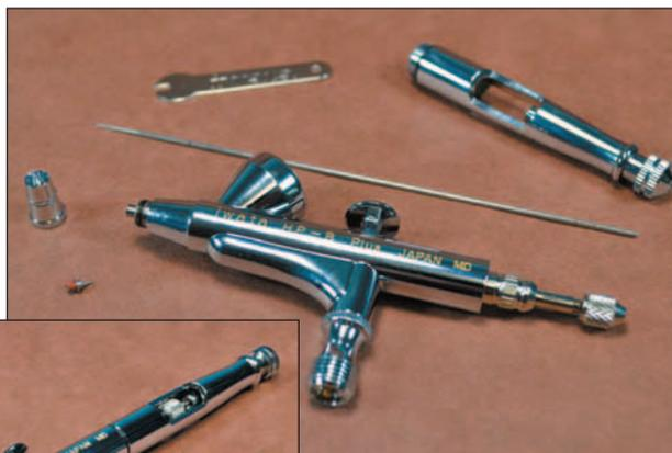
*Left: The Iwata Medea HP-B Plus is a high-quality detail airbrush aimed at the experienced modeler. Above: The unit breaks down easily for cleaning and the components are not affected by modern solvents.*
