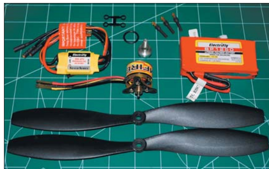
Recommended ElectriFly power accessories include the 28-30-950 brushless outrunner motor, 3S 1250mAh LiPo pack and Silver Series 25A ESC. 3mm-to-5mm adapter and bullet connector adapters are also required.
