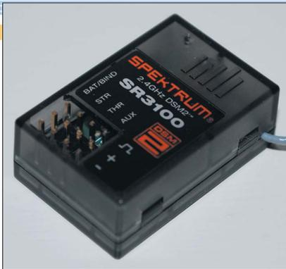
2.4GHz Spektrum SR3100 receiver is a one-piece DSM2 unit. This compact receiver measures only .85 by 1.3 by .48 inches and weighs just .21 ounces. A switch harness and battery holder are included.
