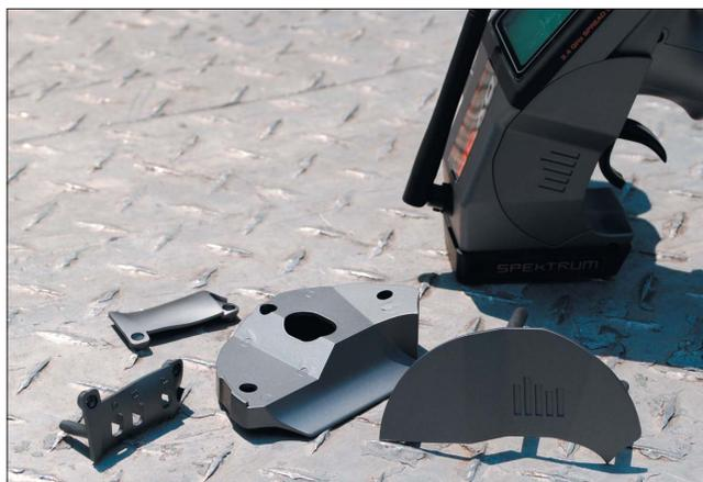
Spektrum DX3R system comes with all the parts needed to convert the transmitter from the standard right-hand operation to left-handed operation. Conversion only takes a few minutes.
