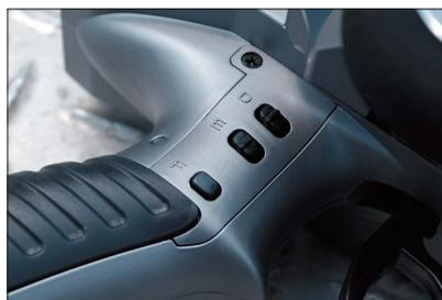
*Roll-and-click programming selector is at the rear side of the transmitter case. On-the-fly driving controls are conveniently located at the thumb position.*
