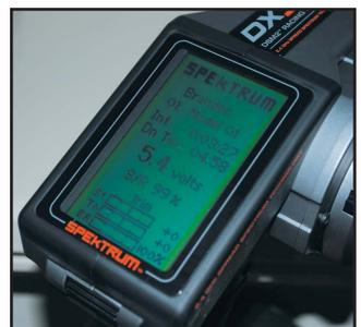
Spektrum's large liquid-crystal display screen features easy-to-read characters for programming convenience, even in bright sunlight. DX3R's programming features are extensive, and include frame rate, exponential, travel, switch assignment, model reset and copy, sub trims, three timer functions and more.
