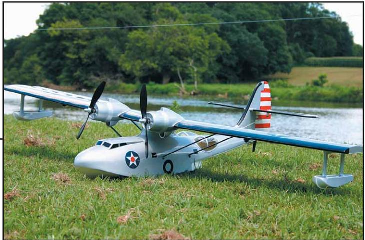
ElectriFly uses two Rimfire brushless outrunner electric motors to power their Catalina, which cuts back on the complexity of the power installation by eliminating the fuel tanks and plumbing, and assuring an ideally matched power curve between the right and left motors.
