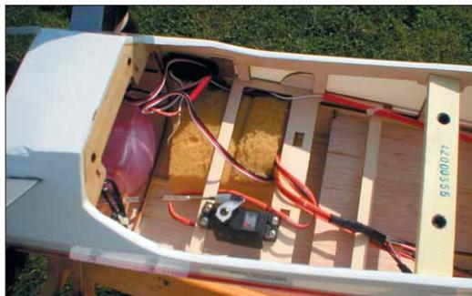
One JR SPORT Standard AIRPAC with two extra ST47 Standard Servos handles the radio requirements of the Seagull Harmon Rocket. Two aileron servos are in the wing, one rudder and two elevator servos are in the tail, and the throttle servo, receiver and battery are mounted inside the cavernous fuselage.
