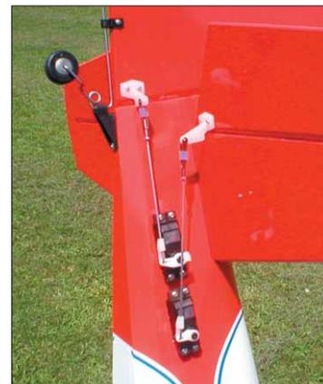
Assembly starts with applying thin CA to the hinges that join the flying surfaces to the control surfaces. Because of the fuselage design, the ailerons, elevators and rudder can all be hinged prior to mounting any of the flying surfaces. The wing consists of two panels that join over a plywood dihedral brace, and
