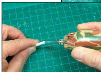
Chassis detail abounds on Trumpeter's Eagle. Prominent are the Hale 2000 GPM pump with the 6-inch side intakes, the drive train, rear differential and suspension. Tom Grossman uses K&S Hobby Drill and the round burr from the accessory pack to hollow the end of an exhaust pipe.
