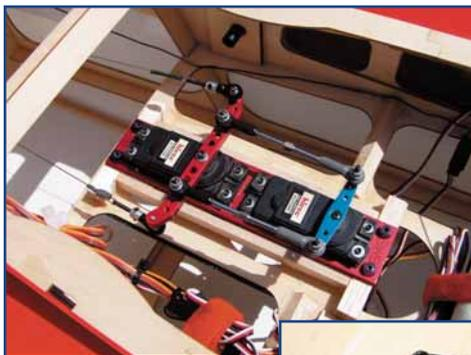
Brandon Wright uses JR 10X transmitter and receiver to direct eight Hitec RCD metal gear servos in his Hangar 9 33 percent Edge 540. Pull-pull control systems and top-notch USA hardware kits assure slop-free surface movement with no flutter. UltraCote strips are used to seal hinge gaps, and Hitec Digital Servo Programmer makes linkage adjustments easy with multiple servos on a single control surface. Hangar 9 offers Edge 540 hardware kits for JR and Futaba servos.
