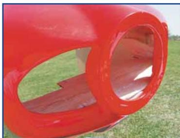
Zenoah GT-80 horizontal twin is one of the recommended engines for the big Edge. Baffles were added inside the fiberglass cowl to direct cooling air over the cylinders during hovering maneuvers. Brandon skipped over the simple spring starter in favor of his powerful Model 4 Mega-Tron electric starter and two NiCD battery packs from Sullivan Products. Diligent planning makes for an excellent engine installation, reliable operation and a long engine service life.
