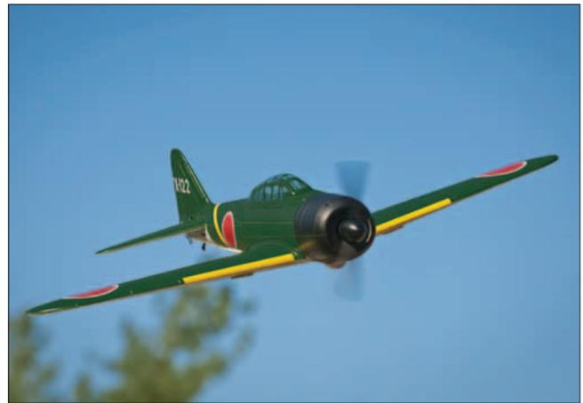
*The Zero's large radial cowl acts like a brake when the throttle is reduced and the bright scheme allows for quick orientation.*
