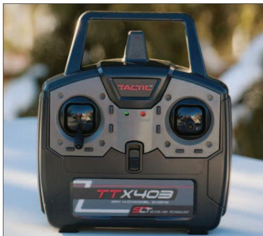
when pressed. The TTX403 is a 4-channel transmitter, but the unit can be set up electronically for basic 3-channel operation (rudder or turning control on the right stick) which makes it a really good match for the AirCore Principle Trainer. Although there is no LED screen to guide a person through programming there are some basic functions like V-Tail and Elevon mixing available which can be accessed simply by moving and pressing the transmit-
