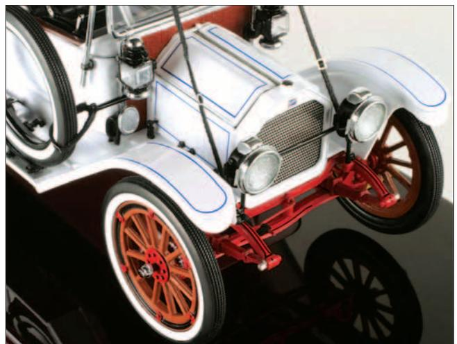
Details such as a photo-etched grill and simulated wood spoke wheels that include the proper speedometer gear add up to an authentic reproduction.
