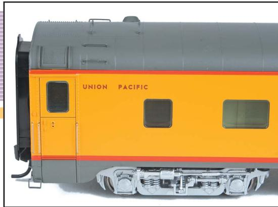
*The vestibule end of the car features wonderful detail including the roof access rungs and handles beside the doors. The GSC Type 42 trucks are very nicely detailed and the prototype's reason for such a smooth ride.*
