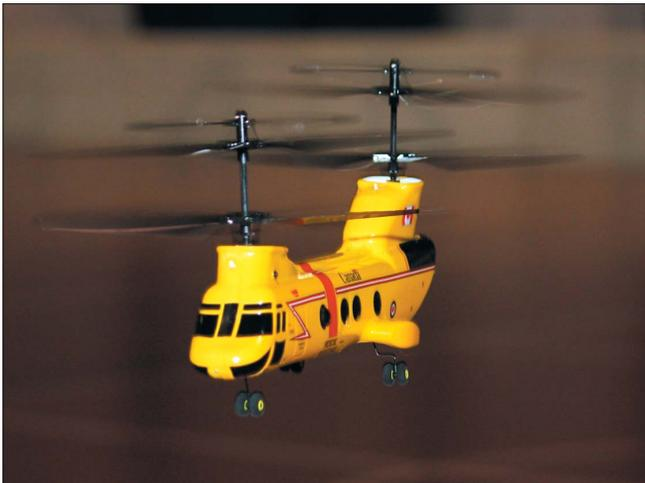
*The Tandem arrangement of the main rotor blades is relatively unique in the world of micro helicopters. Combined with the scale-like appearance of the fuselage, the Tandem offers plenty of eye appeal in flight.*
