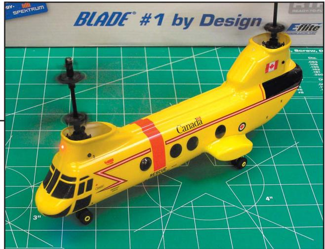
gyros, and servo control units. With the extra motors and electronics the battery was upped from the standard micro 100 mah LiPo to a 250 mah unit. Everything involved with micro flight is a balance of weight and power, and the battery provides a nice combination of light weight and flight time.
