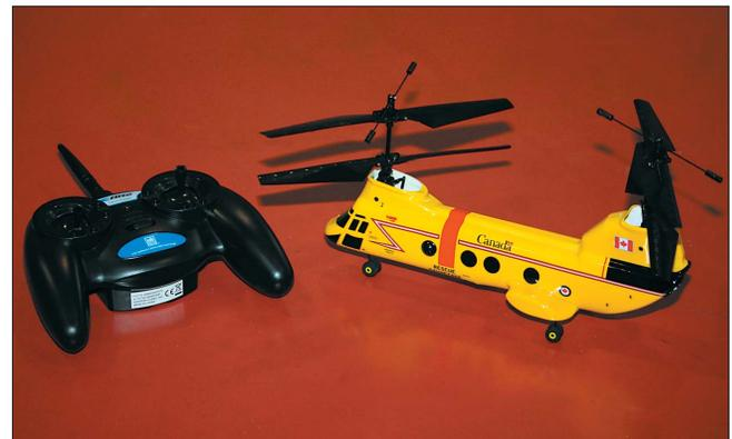
The wheeled landing gear is a departure from the standard strut-and-skid landing gear generally used on micro helicopters.
