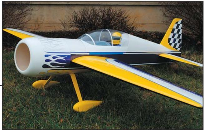
Assembling the Yak 54 begins with an inspection of the kit components. The fuselage is constructed of laser-cut wooden parts with a balsa-covered, foam bottom and turtle deck. The flying surfaces and control surfaces are balsa-sheeted foam with wooden leading and trailing edges, and reinforcement where necessary for strength.
