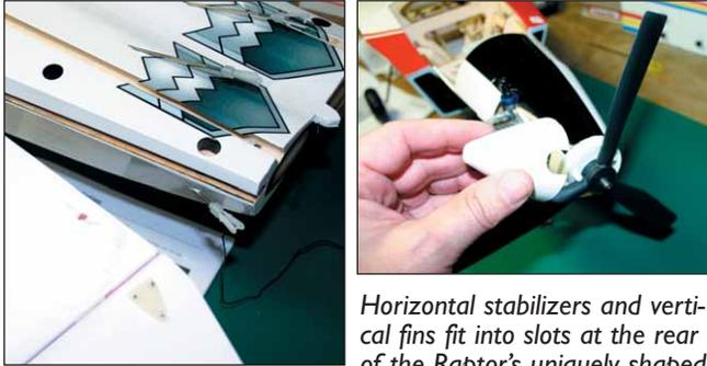
Horizontal stabilizers and vertical fins fit into slots at the rear of the Raptor's uniquely shaped fuselage. Two socket head cap screws secure each component. Assembly concludes with installing the propeller and spinner.
