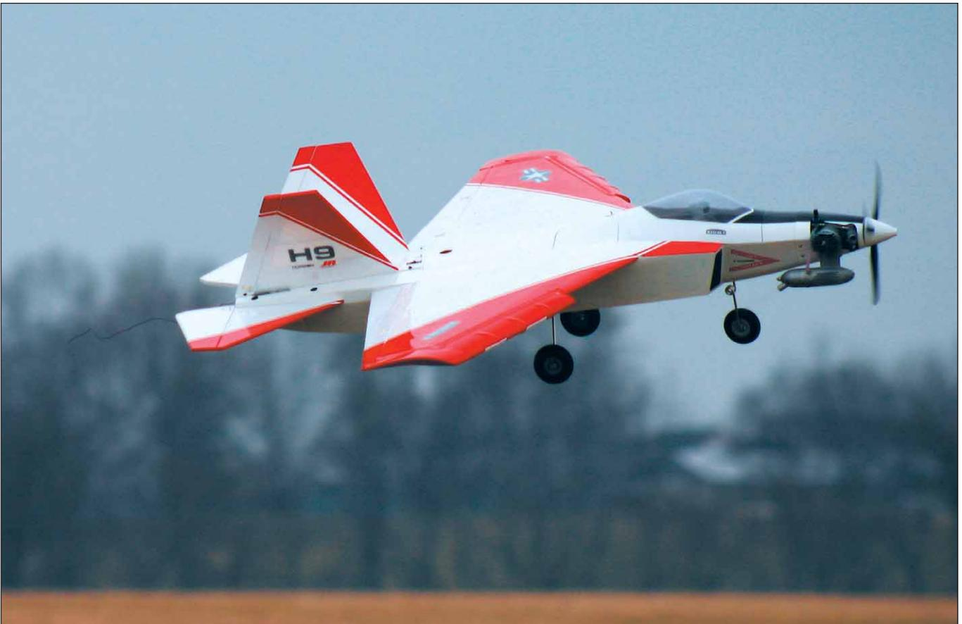
*Yes, it's a trainer. Looks like a jet, flies like a high-wing primary, and will not roll or drop a tip with the droops and extensions installed.*
