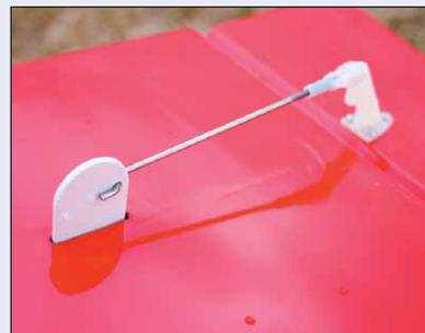
Positionable, mechanical flaps are part of the Hangar 9 F-22 Raptor PTS package. Flaps can be fixed in any of three positions for flight — neutral, half extended or
